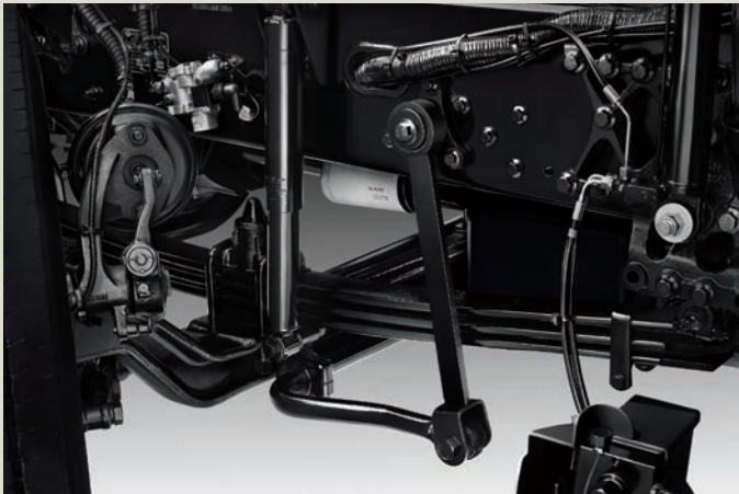
Front suspension (front axle horizontal stabilizer bar + few leaf spring)
